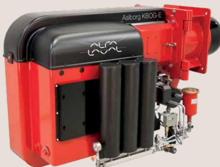
For fuel flexibility, the Alfa Laval Aalborg KBOG-E dual-fuel modulating gas-fired burner is designed for use with small capacity Aalborg OS and OC boilers. It is suitable for firing liquefied natural gas (LNG) as an alternative to heavy fuel oil (HFO) and marine gas oil (MGO) onboard all types of commercial vessels.
