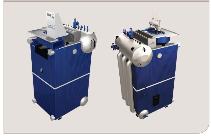
Aalborg D is a standard vertical two-drum boiler. The furnace is built of membrane walls and contains a minimum of refractory. The convection section consists of straight pin tubes with bent pins that provide a high heat transfer coefficient and low pressure loss. Circulation is ensured by downcomers arranged outside the furnace.
