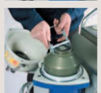
Step 2 Attach the tool and simply lift the separator bowl.
