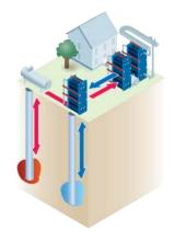
during the winter months (or adverse with cold water used for cooling during the summer). In such applications, aquifers serve as giant thermo bottles. The thermal loss is noticeably low.
