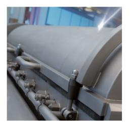
Separation is a key part of the reconditioning stage of this process. By removing any moulds present, separating out the pulp and clarifying the juice, the manufacturer can control the colour, mould content and viscosity of the final product.
