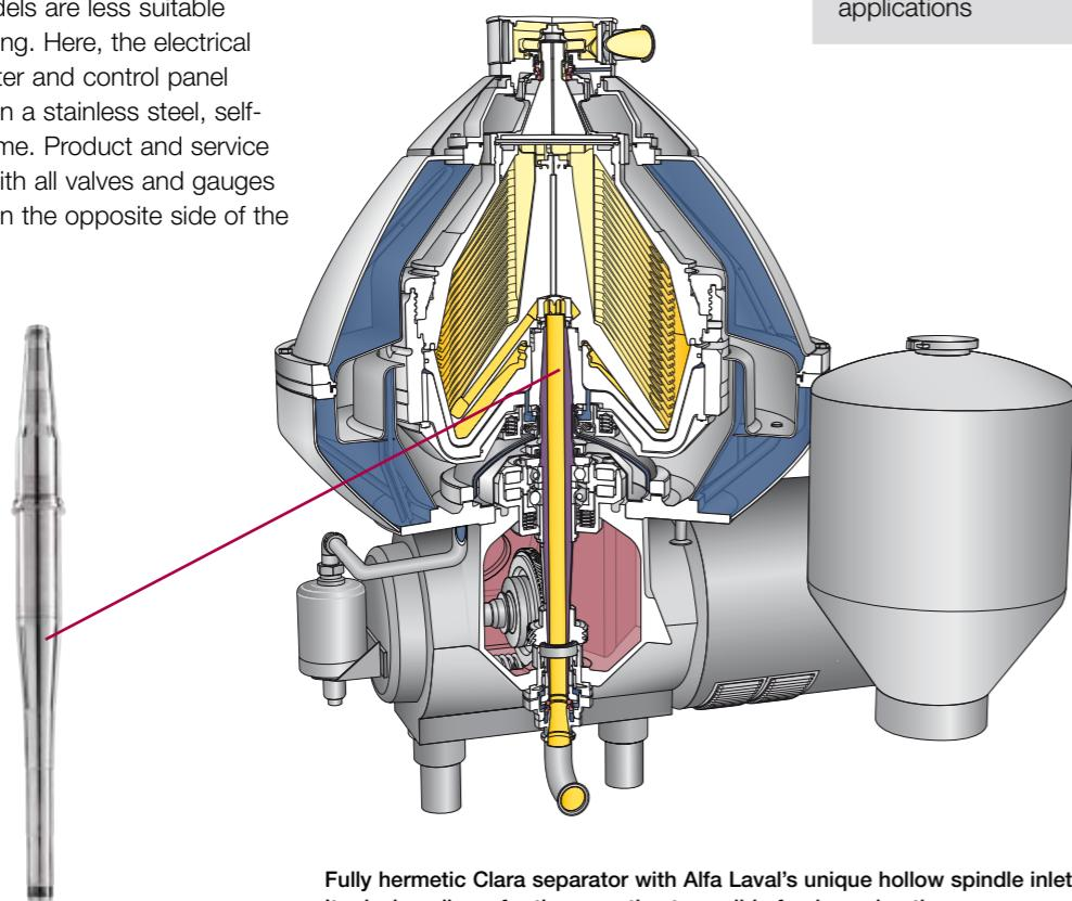
Fully hermetic Clara separator with Alfa Laval's unique hollow spindle inlet. Its design allows for the smoothest possible feed acceleration.
