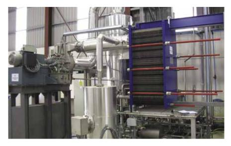
Mechanical vapour recompression system to concentrate effluent. Steam consumption reduced to zero.
