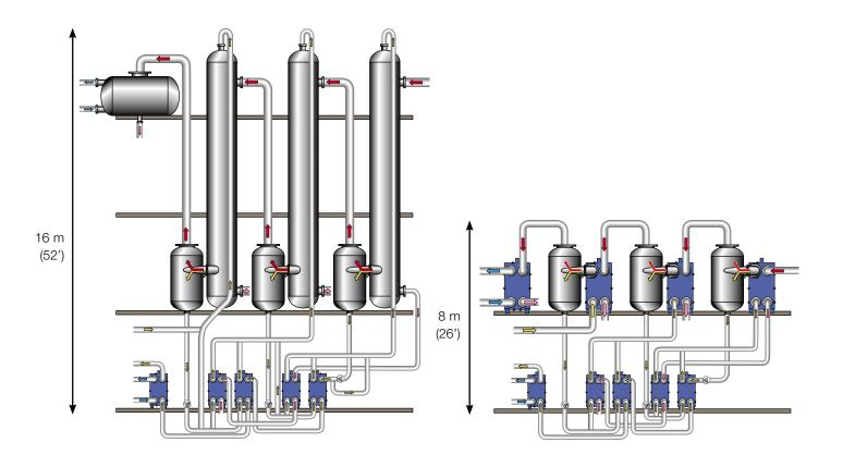
Comparison between shell-and-tube and AlfaVap for a three-effect system that evaporates NaOH from 32 to 50%. The savings in installation costs and space are clearly apparent from the layouts shown above.
