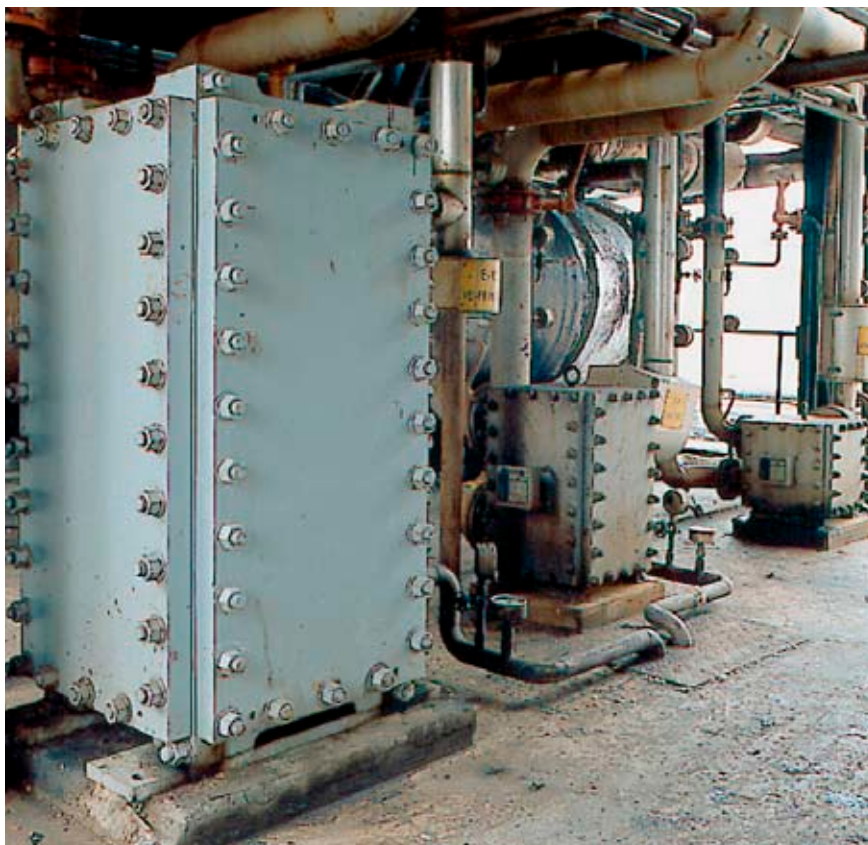
Three Compablocs operating since 1996 as ADU fraction coolers in a northern European bitumen refinery.
