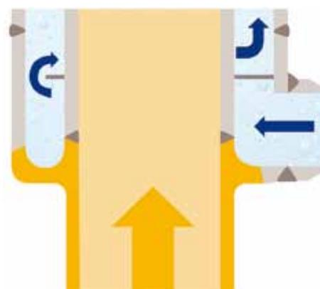
Alfa Laval Olmi's LQE is designed to minimize the residence time of hot gases in the uncooled part of the LQE. Together with highly efficient cooling, this eliminates the need for a thermal sleeve and the risk of ruptures in the inlet.
