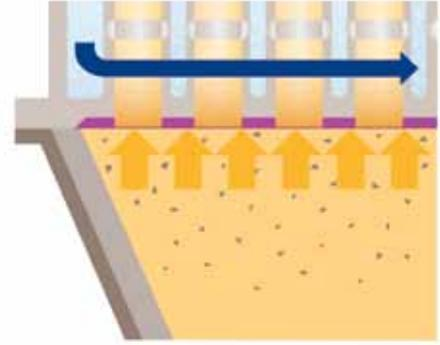
The placement of the welds connecting the tubes to the tubesheet protects them from impacting coke particles, effectively minimizing erosion. The inlet is covered by a layer of Inconel that withstands coke particles in the hot gas. This means there is no need for a distribution device, resulting in a low pressure drop and minimal maintenance costs.
