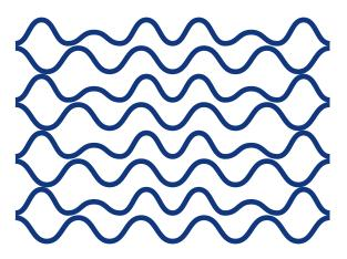
An assymetrical pattern increases the heat transfer efficiency. Alfa Laval offers a number of options suitable for your application.
