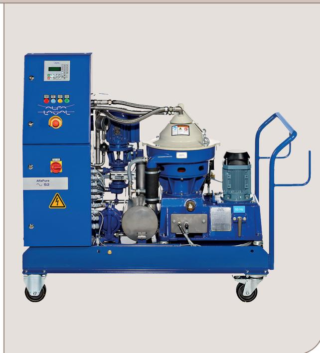
Due to their high speed, disc stack technology, and automatic discharge, Alfa Laval centrifugal separators are an extremely efficient and fast way to remove fine solid particles or liquid contaminants from different kinds of service fluids, using either a two-phase or a three-phase AlfaPure S2 module version.
