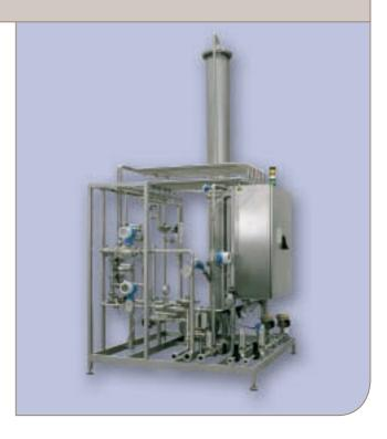
Alternatively, the operator keys in the known and required properties, such as alcohol content or original gravity of the feed and of the end product. The corresponding blending ratio is then automatically calculated and used instead.
