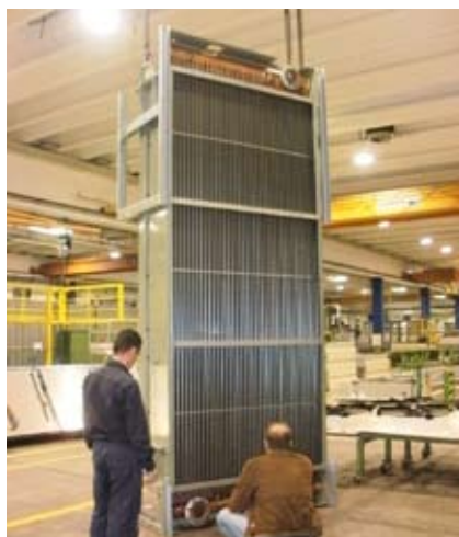
An AlfaBlue transformer oil cooler in the last stage of production at Alfa Laval's air heat exchanger factory in Italy.
