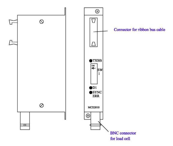
The load cell modules are connected to each other using the supplied cable (10 pole ribbon cable). The TE67X000002029 analog module is connected using the same cable.
