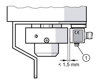
► Check the feedback for the valve states (open and closed). Indication via LED and visual pointer position.
