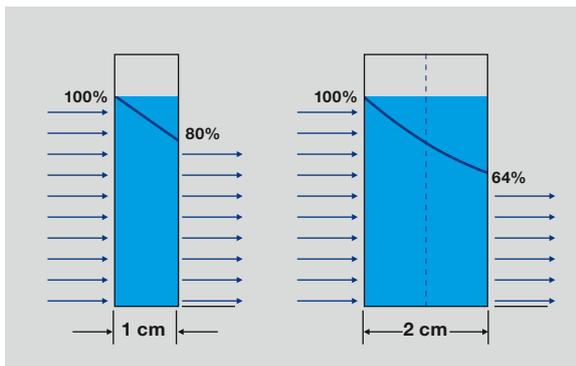
An example of UV transmittance (80%), showing the decrease in light intensity with distance from the source. Note the limited light remaining after passing through 2 cm of unclear water.
