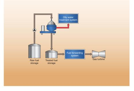
The purified oil is pumped to a treated fuel storage tank prior to being forwarded to the gas turbine or diesel engine.
