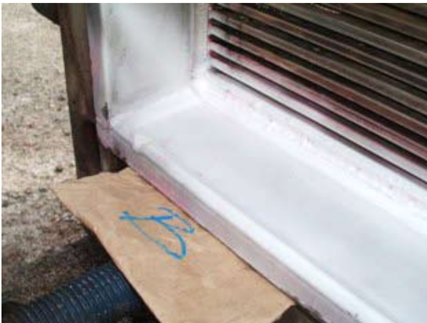
Here the result of the dye-penetrant test after a corner weld has been TIG repaired.
